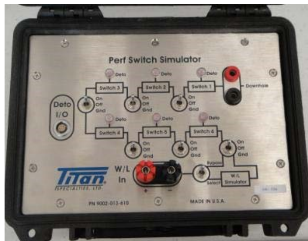
Figure 6 Perf Switch and Wireline Simulator Panel
